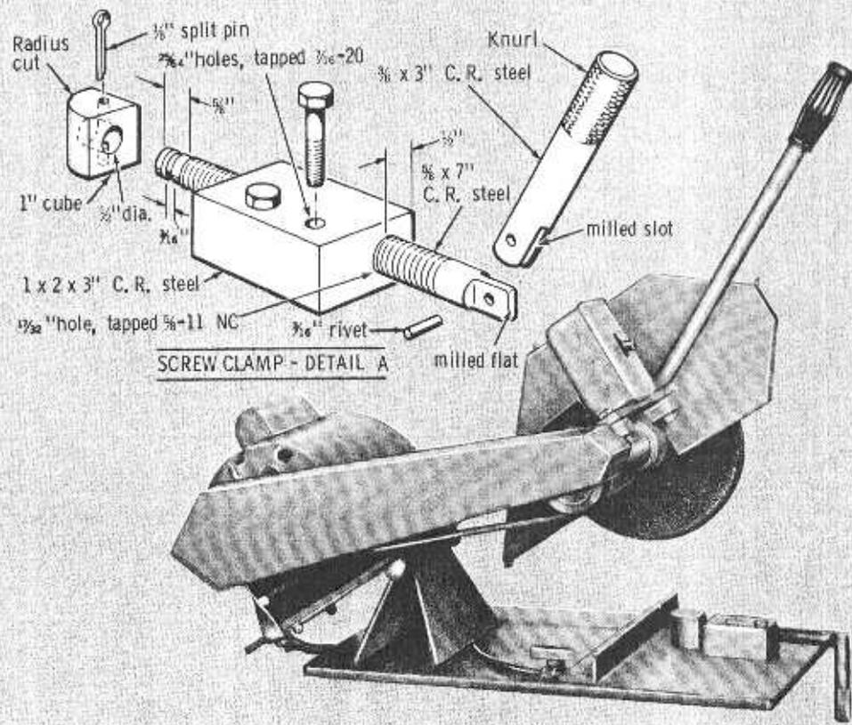
the weight of the motor will only slightly overbalance the weight of the arbor end of the assembly. For this reason, make the hinge, but do not weld to either plate until after the mandrel, blade, guards, handle and switchbox are at least temporarily mounted.
