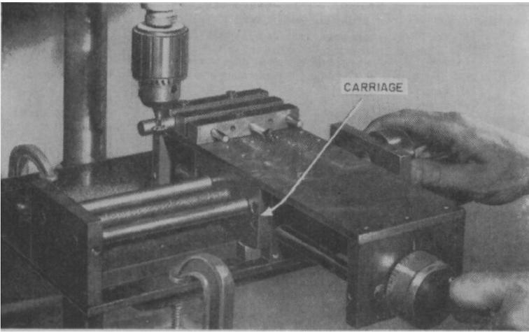
Cutting a keyway in a piece of cold-rolled shafting is easy with the compound table. In this set-up, depth of the cut is controlled with the left hand lead-screw, while the work is advanced with the right hand lead-screw.
