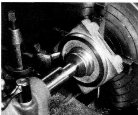
**OTHER TYPE** of vise casting is first center-drilled for tailstock support. Then the compound is swung to 30° for turning the post to a duplicate of the one on the cross slide. Facing (above) completes work on this side.
