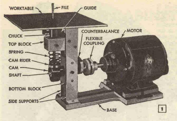
Both modelmakers and die makers will like the precise internal and external filing this machine can do on a wide variety of small intricate work. It uses the standard machine file
