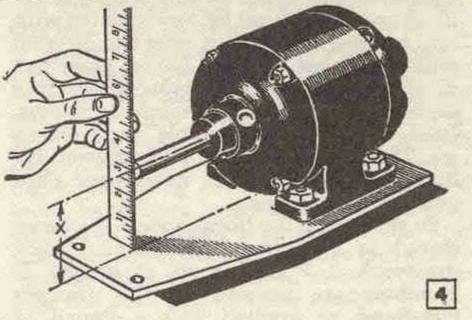
Above, be sure of this dimension as it will vary with different motors. Below, standard machine files with ¼-in. round shanks are used. By fitting an interchangeable chuck, machine makes a speedy jigsaw
