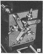
Your lathe will become a better tool with this center rest. Adjustment screws give delicate control over the centering of the work, and jam nuts provide a nonslip grip once the proper adjustment has been made
