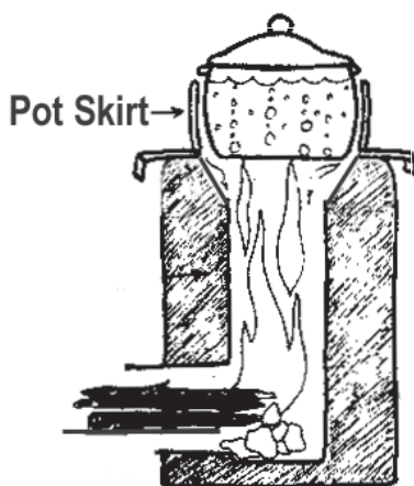
Figure 2 - Appropriate Use of Pot Skirt
