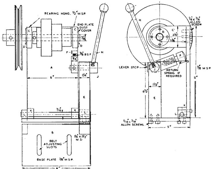
which forms a hinge pin, thus allowing the entire backplate and bearing housing to swing freely about this point. Its movement is controlled by a thrust member with a screwed adjustable head, F, which is mounted on the cam spindle, J, and acts as a toggle against the face of the backplate A.
