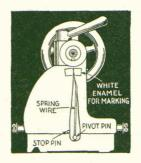
ters without loss of time if this indicator is used. It consists of a sheetmetal pointer pivoted to a pin in the lathe bed, and a length of spring wire, which is fastened rigidly in the pin and wrapped around the pointer. The
