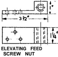
ELEVATING FEED SCREW NUT
