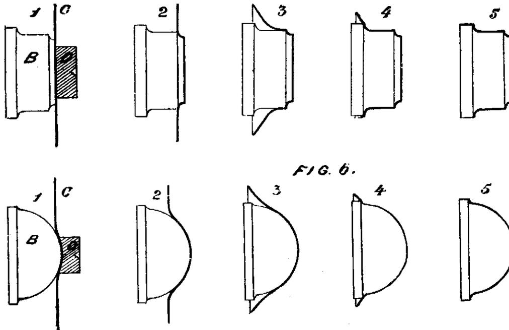
The material will get easier to move as the part is closer to completion (unless it has work hardened too much in which case it should be annealed), but patience must be exercised so that the fully formed part requires a minimum of finishing. Just keep repeating the same smooth fluid strokes from inside to outside until the part is seated and then start to move the material from the outside in, but always try to leave a bump or rib to protect against warping and over-stretching.
