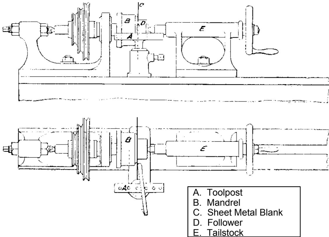
Custom grooving or forming tools can be easily fabricated and even mounted directly to the crossfeed if it is a simple form. Spinning with the tool attached to the crossfeed limits one's ability to feel the material and form it smoothly. A compromise, for example, is swaging where a rolling tool forms the metal without a buildup of friction (i.e. bad surface finish).
