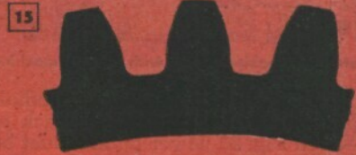
5 DIAMETRAL PITCH 0.6283 CIRCULAR PITCH
