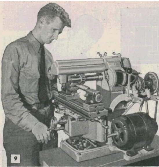
Accurate spacing for milling the teeth of an angular cutter is accomplished by mounting the work in a chuck fastened to an indexing center which, in turn, is bolted to an indexing table. Angular cutter is then heat-treated and ground
