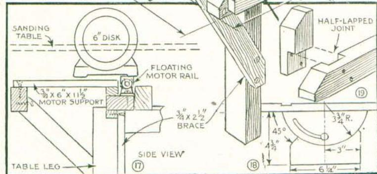
and the blade. A lock pin fitted through the front trunnion permits the table to be returned quickly to a horizontal position without need for checking the angle each time.
